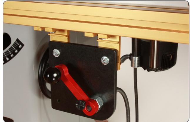
Add a large flat washer to each of the 3/8-16 x 3/4" hex bolts and thread a 3/8-16 rectangular nut onto the end of each bolt. Slide the rectangular nut on each of the bolt assemblies into the T-slot located on the underside of your INCRA TS System's front rail and position the bolts close to your router, **Fig. 1**. (You'll be able to adjust the final position after full assembly.)
