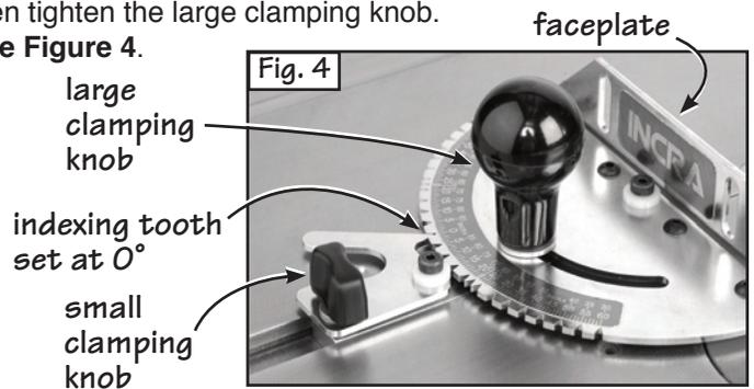
❷ Using the supplied 1/8" hex key, loosen the (4) button head fasteners that secure the faceplate to the protractor, and depending on your application, square the faceplate to the blade, miter slot, sanding belt, etc. **NOTE:** When squaring to a saw blade (see **Figure 5**), use a reliable square for this important alignment. Securely retighten the (4) button head fasteners to complete the alignment.
