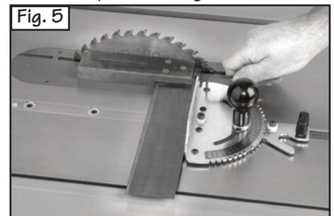
This important one-time adjustment prepares your INCRA Miter V27 for perfect angles at all other indexing tooth positions. Verify the accuracy of your alignment with a test cut, and re-align if the cut is not exactly 90 degrees.
