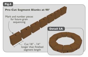
the blade, then lock the platform in place with the Build-It Clamp. Now simply place each blank's reference edge against the fence, nesting the previous cut against the end of the toggle clamp platform and engage the toggle clamp to cut a perfect finished segment.
